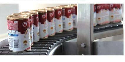
The Single lane Spiral Conveyor is modular built with a small footprint to save floor space. These spirals are easy to install as they are pre-assembled before delivery.
